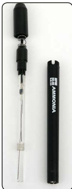
The YSI TruLine Ammonia ISE. A pH electrode is placed inside an outer membrane module that is only permeable to ammonia gas.
