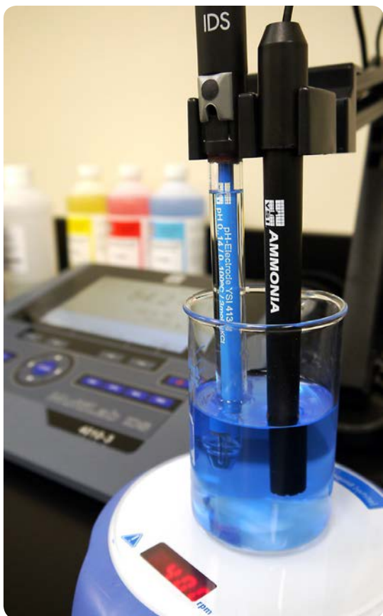
Ideal set-up for calibration. A stir plate, 150 mL glass beaker, temperature sensor (e.g. from pH electrode), ISE instrument, and ISA are all used.
