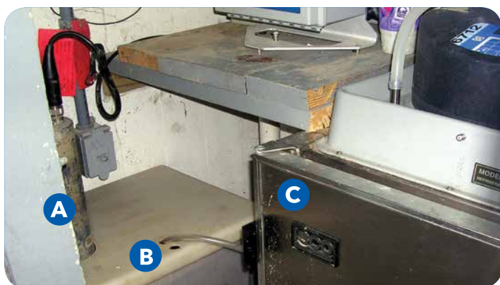
Figure 2. Contents of gage station, including A) sonde, B) sidestream vessel, C) auto sampler. Web-based data collection platform not shown.
