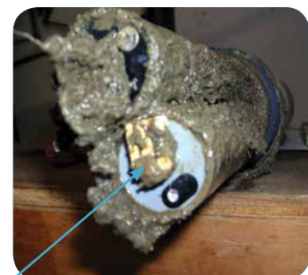
Figure 4. Sediment fouling on sensors
