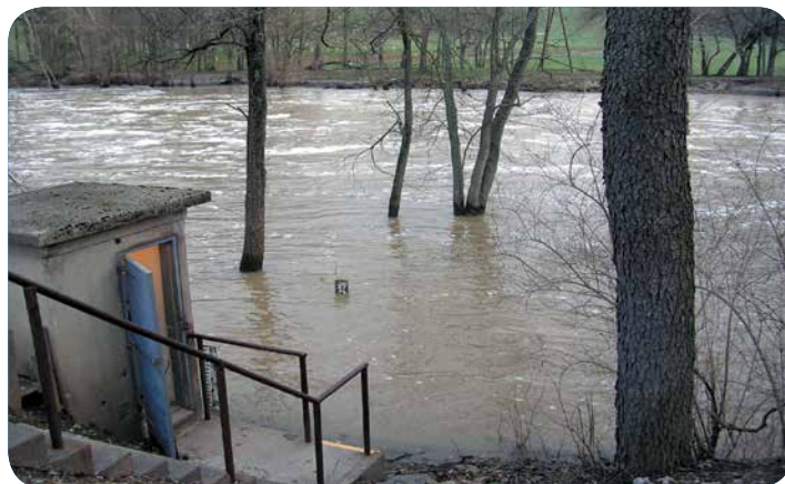
Figure 1b. Gage station at high flow/high turbidity. Sidestream methodology prevents the water quality sensors from getting damaged during flood events.
