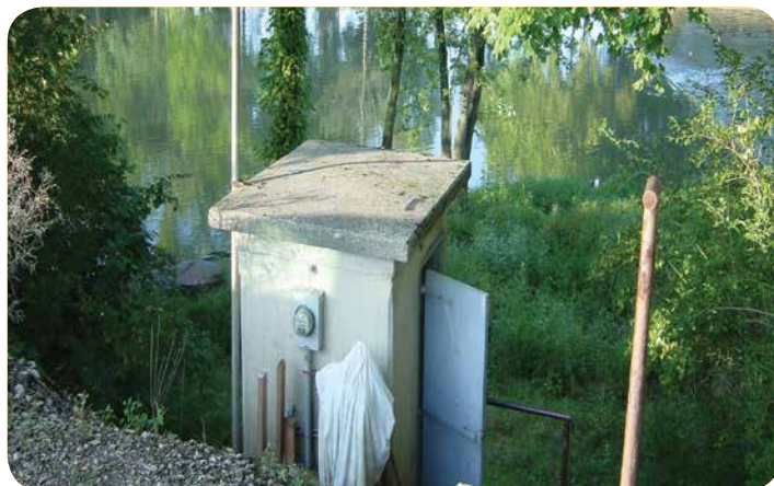
Figure 1a. Typical gage station for sidestream monitoring of rivers, during normal flow.
