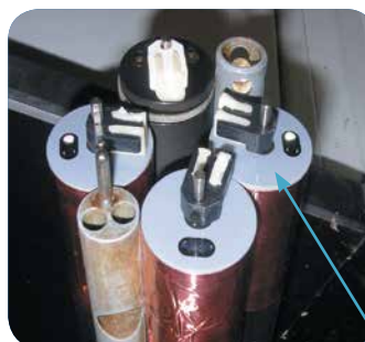
Figure 3. Sensors in sonde
