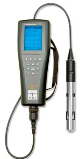
The YSI Pro Plus was used during the studies to acquire fast, simple field measurements of nitrate nitrogen.
