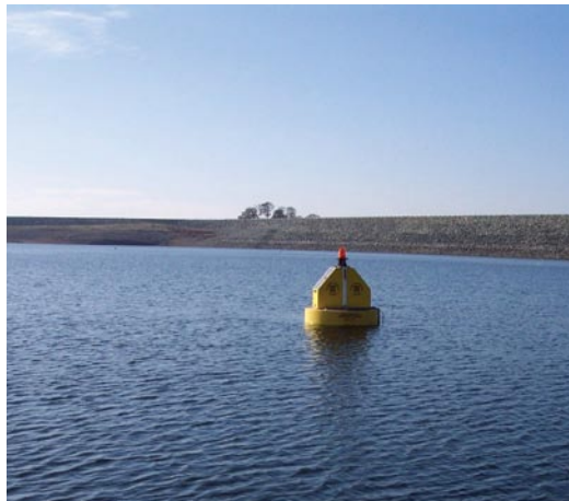
A YSI Vertical Profiling System takes continuous water quality measurements in the Camanche Reservoir. The sonde under the buoy is programmed to automatically collect readings at set intervals throughout the water column.
