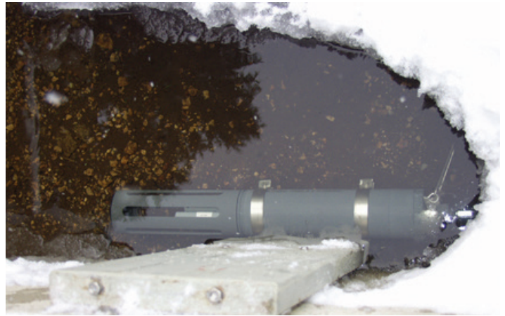
YSI multiparameter sonde deployed under the ice.
