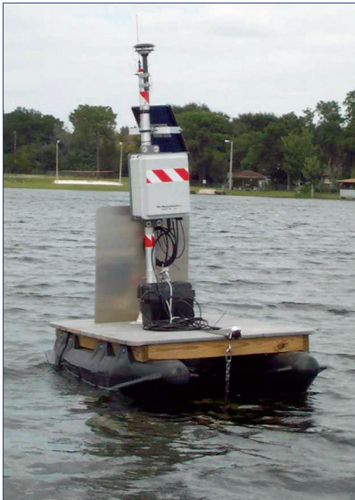
Figure 1 YSI Data Acquisition System deployed on Bear Lake near Semi- nole County, Florida
