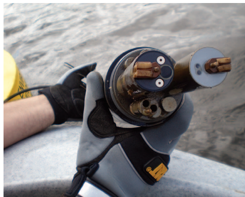
Autonomous water quality monitoring buoy in the River Tyne; dissolved oxygen, turbidity, and temperature sensors on a YSI sonde attached to the buoy
