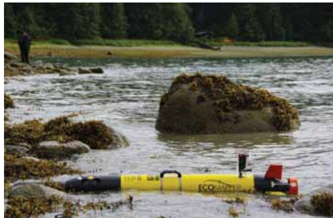
YSI EcoMapper AUV collected bathymetric data across two lakes in a remote Alaskan mountain region
