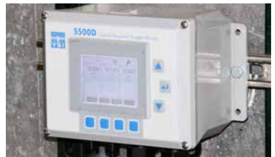
YSI 5500D Optical Dissolved Oxygen Monitor for continuous monitoring and control
