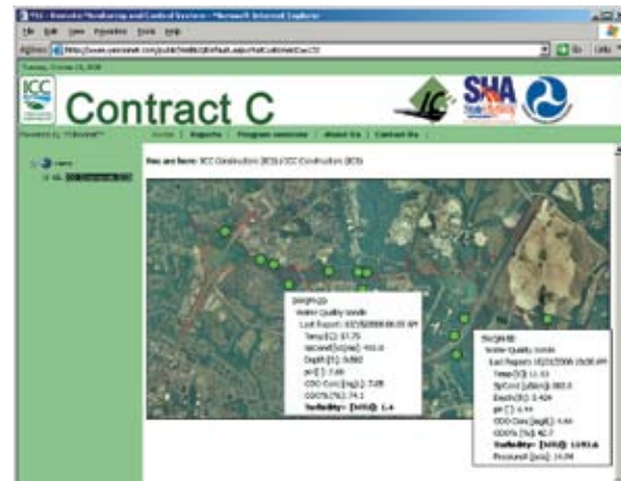
Above: Data from water quality monitoring stations can be viewed in real-time via the web. Below: Rainfall and subsequent runoff into stream created a turbidity spike captured by real-time monitoring.
