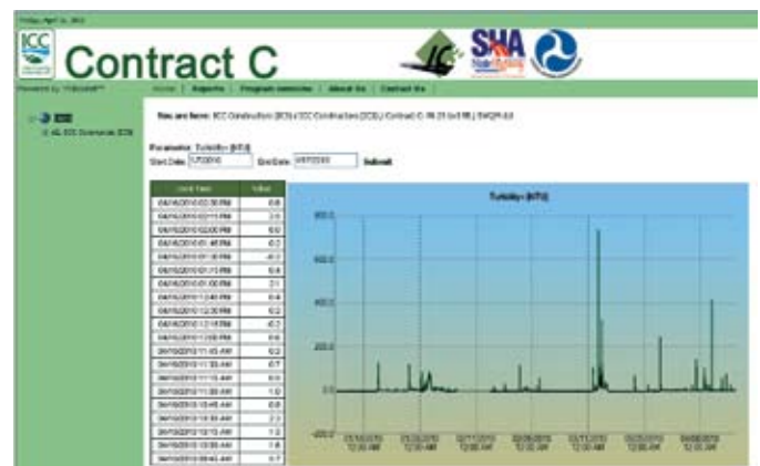
Above: Data from water quality monitoring stations can be viewed in real-time via the web. Below: Rainfall and subsequent runoff into stream created a turbidity spike captured by real-time monitoring.
