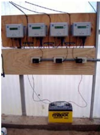
Each raceway was equipped with a YSI 5200 continuous monitor, logging DO and temperature every 5 minutes.
