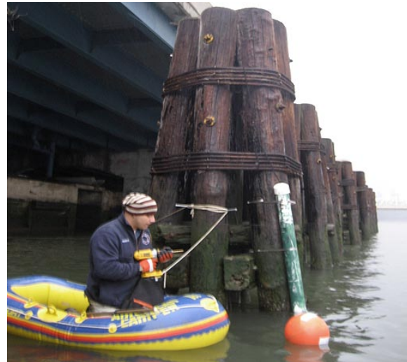
Students at the Frederick Douglass Academy in New York continuously monitor the Harlem River using a YSI 600OMS sonde. The sonde is positioned inside a PVC tube and attached to a bridge piling.
