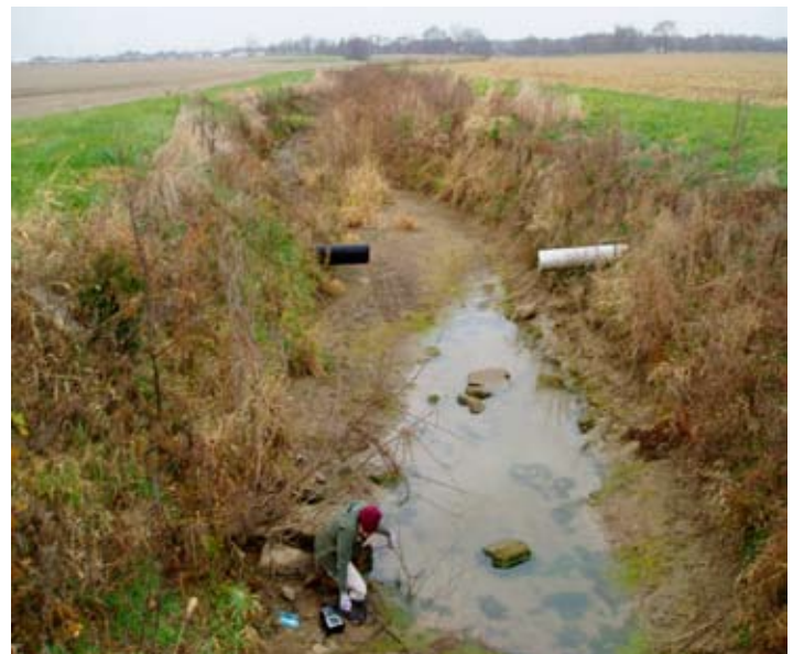
BCWP personnel conducting surface water quality monitoring with a YSI 556 handheld multiparameter instrument.
