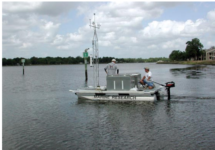
Above: Solar-charged batteries, flow cells, and satellite transmitter allow the equipment on a mobile MARVIN system to maintain around-the-clock data collection schedule with maintenance just twice per month.
