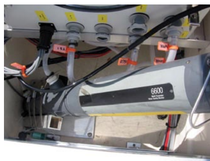
Below: Solenoid-governed water samples drawn from two or three depths pass through flow cells for monitoring, minimizing biofouling and increasing service life. An automatic wiper on this YSI 6600EDS multiparameter sonde also reduces maintenance needs.
