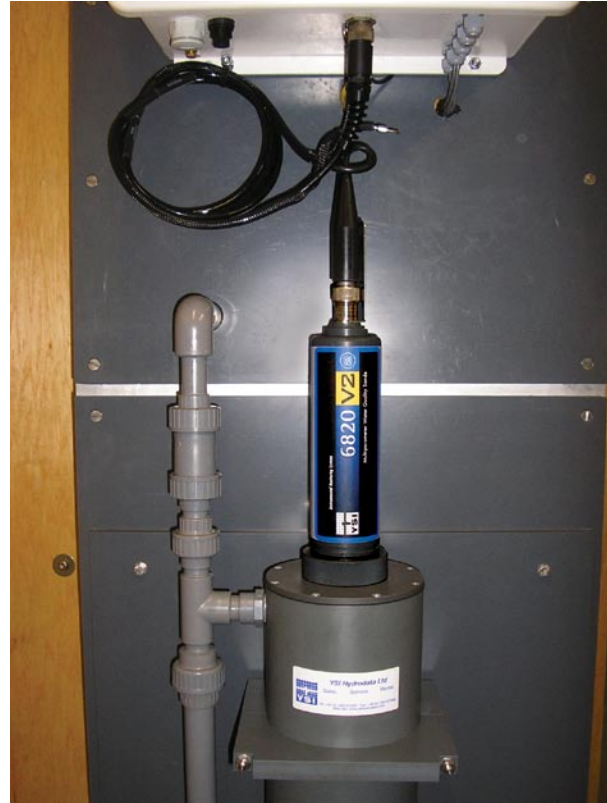
A YSI sonde contains multiple sensors for water quality parameters. To collect data, water is pumped through a single chamber past the sensors.
