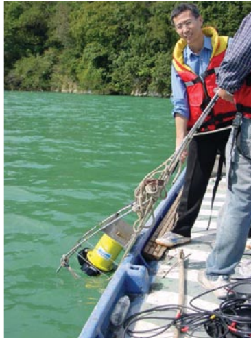
Above: Bergius Su and his team used a SonTek/YSI acoustic Doppler velocimeter to identify optimum sites for the profiling systems deployed to protect Shimen Reservoir's water treatment plant.
