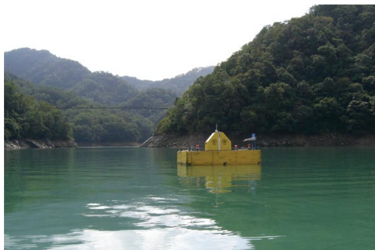
Below: Autonomous vertical profiling systems mounted to pontoons help managers of the Reservoir track turbidity throughout the water column.
