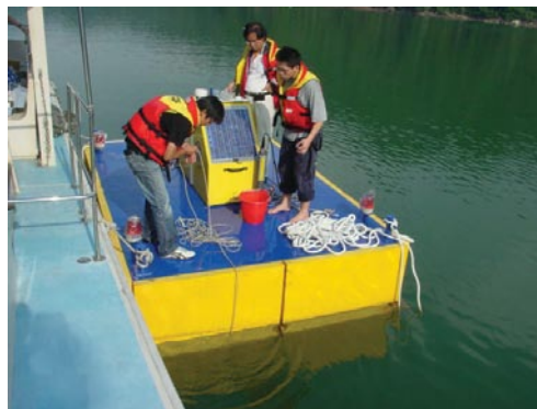
Below: Each vertical profiling system features a YSI 6600EDS multiparameter sonde that measures turbidity, chlorophyll, pH, and dissolved oxygen every 5 meters from surface to bottom.
