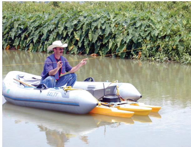
David Murdoch of LCRA deploys a trimaran-mounted RiverSurveyor to measure flow throughout the vertical water column. In obstructed reaches, the instrument's stationary software delivers excellent data to a simple, intuitive interface, says Murdoch's colleague, Keith Ging.
