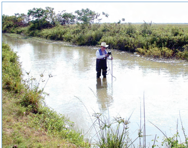
Lower Colorado River Authority senior hydrologist Keith Ging uses a FlowTracker acoustic Doppler velocimeter to gather fast, accurate data for flow studies.
