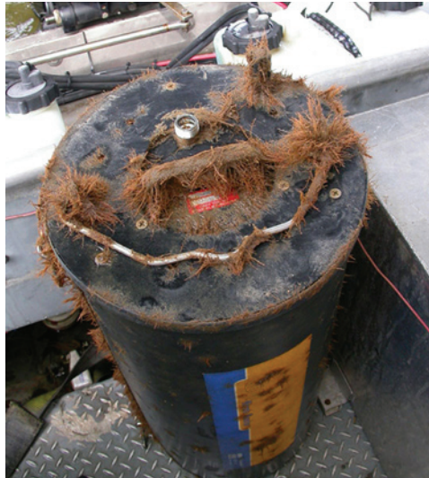
Biofouling on a YSI 9600 after deployment at Rigolets, Highway 90 near Slidell, Louisiana.
