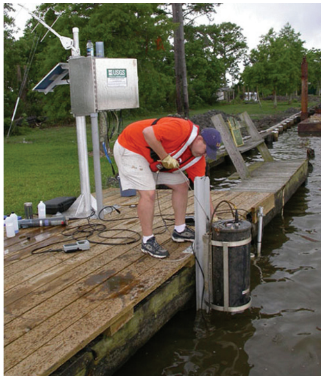
Deployment of the YSI 9600 at Pass Manchac, Turtle Cove near Ponchatoula, Louisiana.
