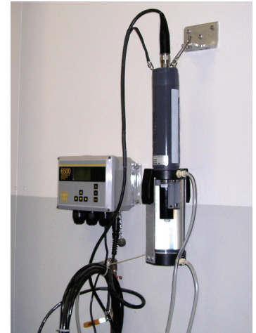
YSI 6920DW deployed at a water tower in Columbus, Ohio. The instrument, used in conjunction with a flow cell and a YSI 6500 Process Monitor, continuously monitors drinking water quality.
