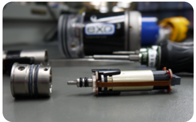
Annual Wiper service is critical to anti-fouling protection
