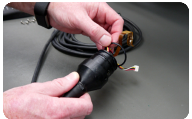
Cable/probe assembly seal replacement
