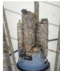
30-day comparison of sondes deployed side by side anti-fouling biofouling
