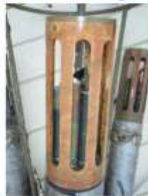
30-day comparison of sondes deployed side by side anti-fouling biofouling
