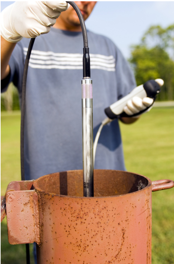
The YSI Level Scout provides highly accurate pressure and water level measurements.
