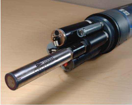
YSI 6600 water quality sonde with adapted Turner hydrocarbon sensor monitors oil in polluted waters, shipping channels, and mines
