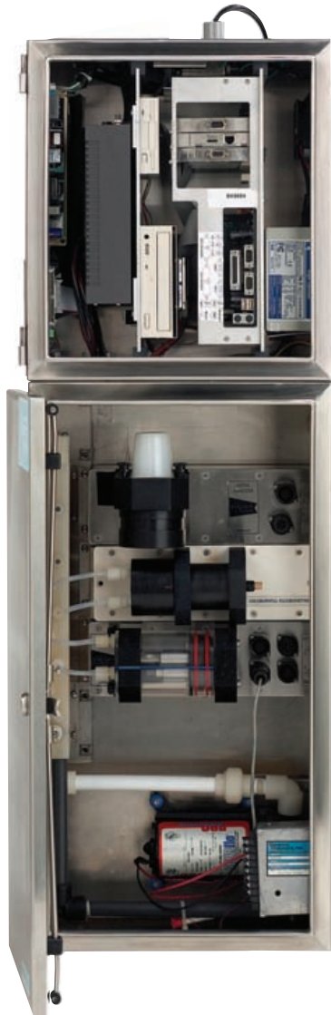
Standard SeaKeeper 1000 with computer controller (top), and flow-through sampling system (bottom). Data is displayed on a local computer and transmitted to National Weather Services worldwide.
