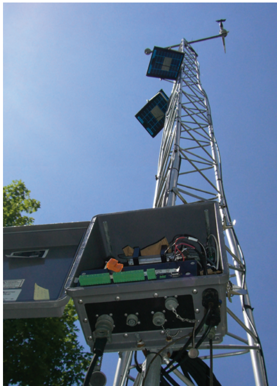
Met sensors and accessories configured on a land-based tower.
