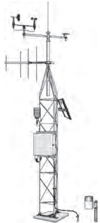
Met sensors and accessories configured on a land-based tower.
