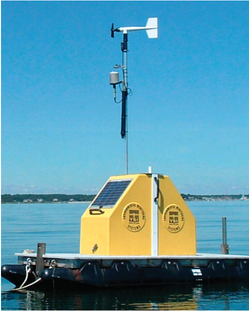
YSI Vertical Profiling System with Meteorological Sensor Suite, deployed in drinking water reservoir. Wind direction (top), speed, and relative humidity sensors are mounted on the mast.
