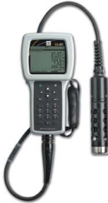
YSI 556 handheld multiparameter instrument.
