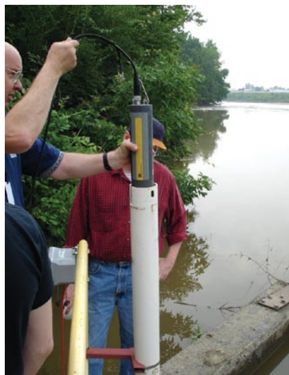
A YSI Vertical Profiling System (above) and 6600 sonde (below) are deployed in on-stream reservoirs in order to collect real-time source water data
