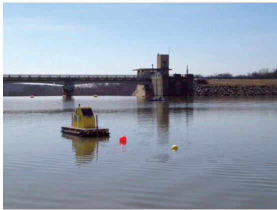
A YSI Vertical Profiling System (above) and 6600 sonde (below) are deployed in on-stream reservoirs in order to collect real-time source water data
