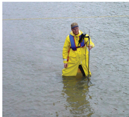
John Roberts of LCRA's Hydromet Operations group used FlowTracker acoustic Doppler velocimeters to check hydroturbine ratings near a dam.
