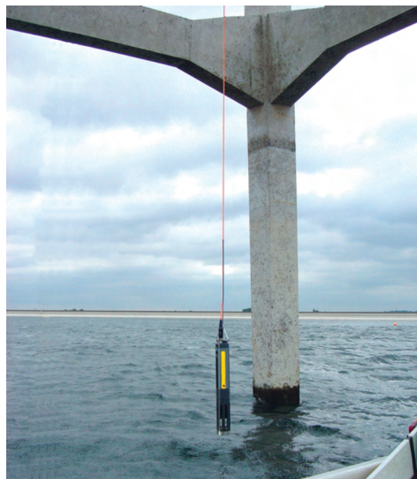
A YSI multiparameter water quality sonde is fixed to, and lowered from, a tower in the Queen Mother Reservoir. It will profile the entire water column of the reservoir.
