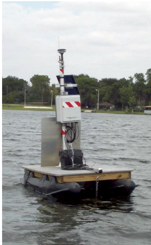
Figure 1. YSI 6200 Data Acquisition System deployed on Bear Lake near Seminole County, Florida.
