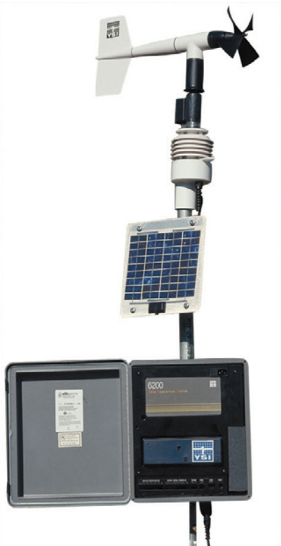
The YSI 6200 data acquisition system provides remote data access and real-time readings.
