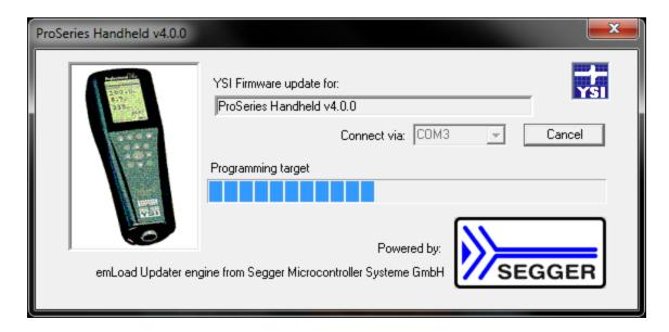
11. The update process will take approximately 5 minutes. When the update is complete, the application will display "Target updated successfully". You may exit the Updater program and disconnect the instrument from the saddle.
