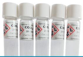
COD vials must be disposed of properly in order to safely dispose of the mercury inherent to the test.
