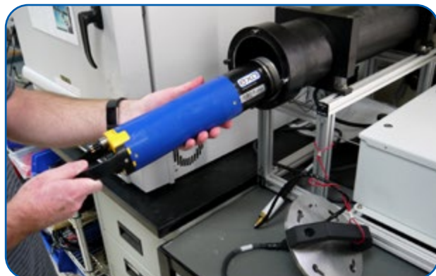
Factory pressure chamber tests leak resistance up to 250m simulated depth
