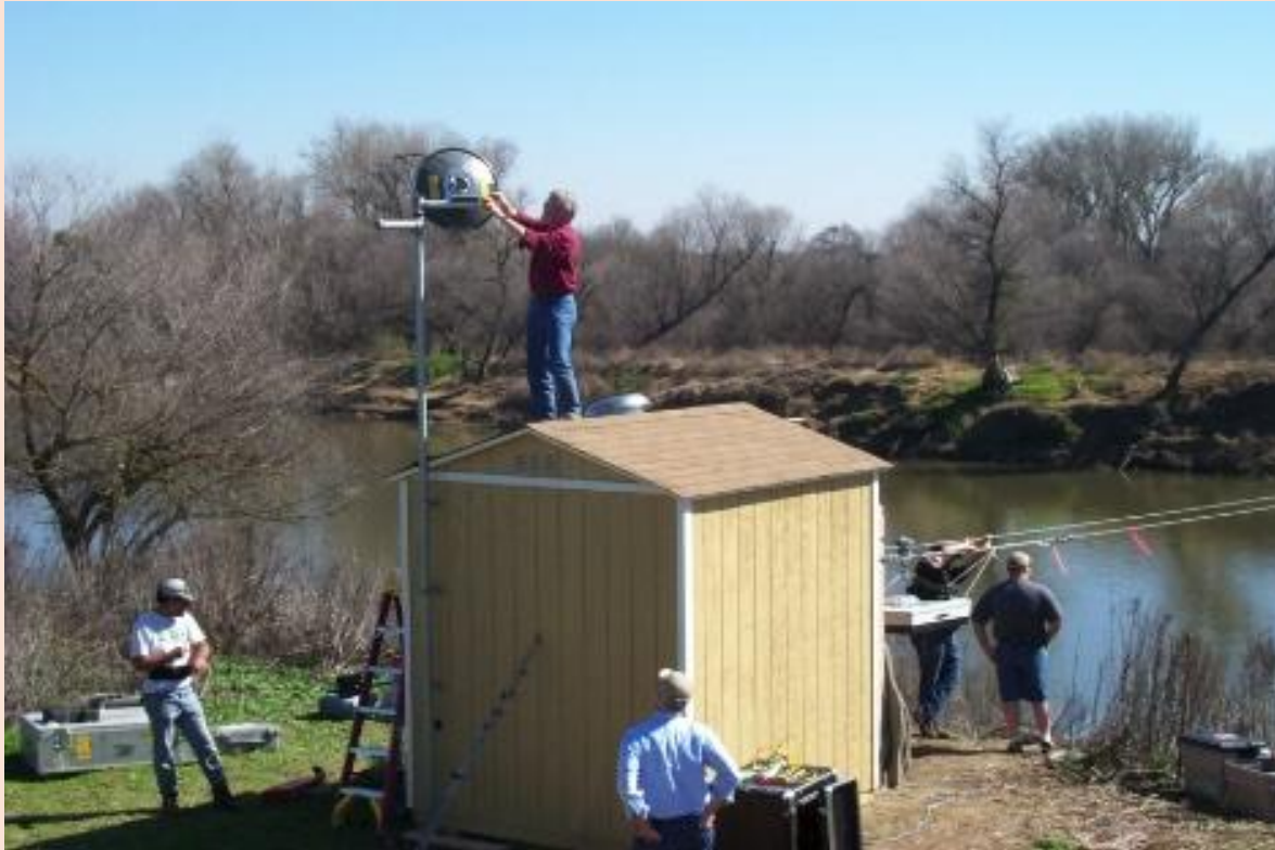
Bragg-scatter surface-velocity radar antenna and ground-penetrating radar, San Joaquin at Vernalis, CA (2002)
