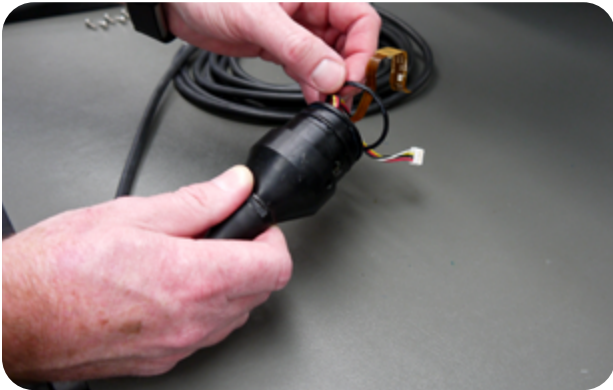
Cable and probe assembly seal replacement
