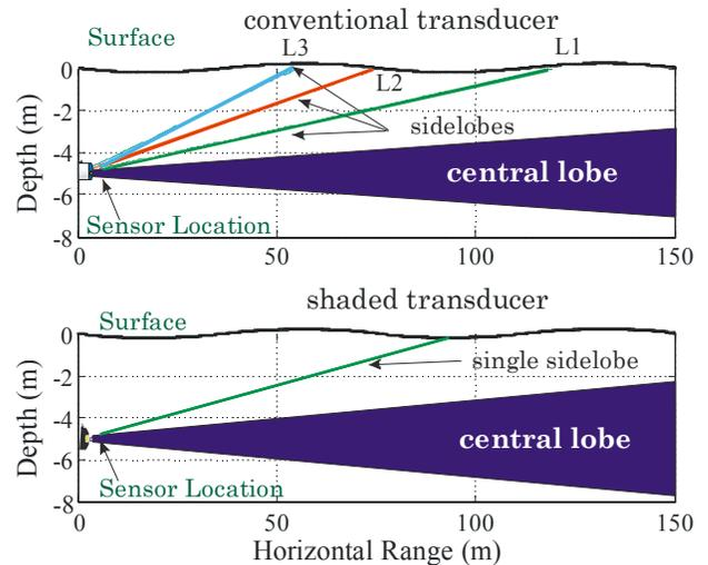
Figure 8: Effects of side lobe suppression on practical aspect ratio in horizontal current profiling. In a conventional design (top plane) the maximum profiling range is limited to approximately 55 m due to interference from the L3 side-lobe. The shaded design (bottom plane) achieves approximately 85 m horizontal range due to a much narrower beam pattern as a result of side lobe suppression. Practical aspect ratio is increased by more than 50%
