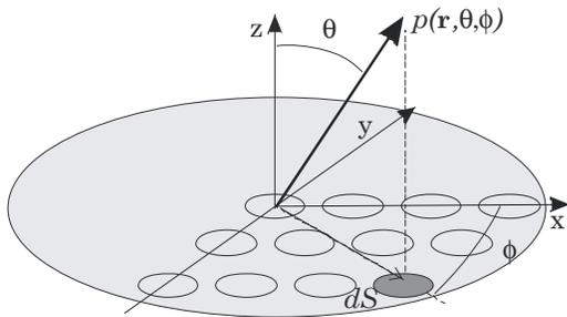
Figure 2: Geometry used for computing directivity pattern using a finite element numerical model. The overall pressure field is computed as a superposition of contributions from individual elements on the transducer face (x-y plane). Adapted after [5].
