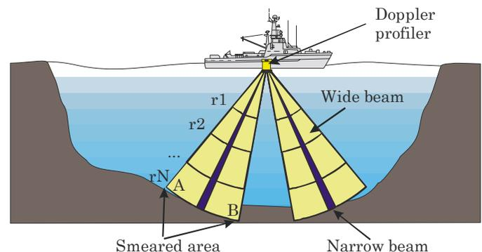
Figure 1: Diagram of acoustic Doppler current profiling from a vessel. Directional Doppler profiling transducers feature beam widths between  $1^\circ$  and  $6^\circ$  (depicted in dark blue), which allows precise positioning of the insonified volume. Wider beams (shown in light yellow) cause increasing spatial smearing with increasing range, which severely limits spatial resolution and induces potential velocity bias, compared to the narrow beam transducers.
