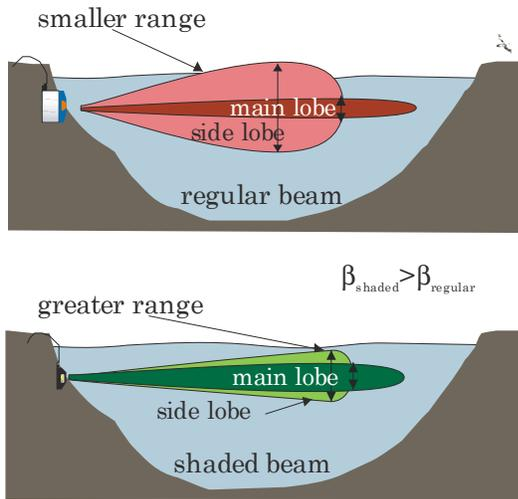
Figure 7: A sketch of transducer shading effects on the maximum achievable range in side-looking profiling application. Note that while the main lobe of the regular design is narrower, the width of the first side lobe is quite large in comparison (top plane). Conversely, the shaded transducer (bottom plane) shows a much narrower first side lobe, making its effective beam width for the horizontal application quite small in comparison. This is critical in achieving larger aspect ratio  $\beta$ .
