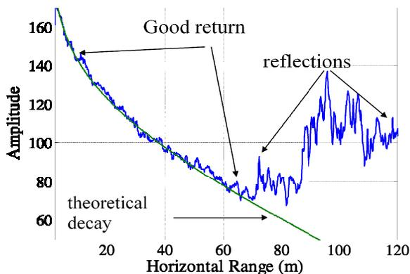
Figure 9: Acoustic signal strength profile as a function of range collected with a software utility BeamCheck. Echo return is free from reflections up to 70-m range and agrees well with the theoretical signal decay, computed according to [3]. Boundary reflections dominate signal return between 70m and 120m. The strongest reflection peak exceeds the ambient signal level by almost 40dB. Data were collected with a 500-kHz horizontal profiler.
