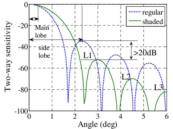
Figure 3: Modeled shaded transducer sensitivity demonstrating side lobe reduction (dashed line) when compared to a regular transducer design (solid line). First side lobe L1 is suppressed by  $>20$ dB (100 times); higher order side lobes (L2 and L3) are practically nonexistent. The overall transducer directivity is improved by  $\sim 60\%$ , when referenced to  $-50$ dB level.
