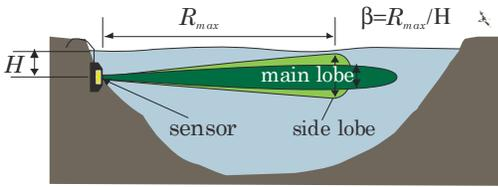
Figure 6: Diagram of a typical Doppler sensor installation in horizontal current profiling applications.  $R_{max}$  denoted maximum achieved horizontal profiling range, while  $H$  is the installation depth below mean water level. Dark and light green shapes depict center lobe and first transducer side lobe respectively.
