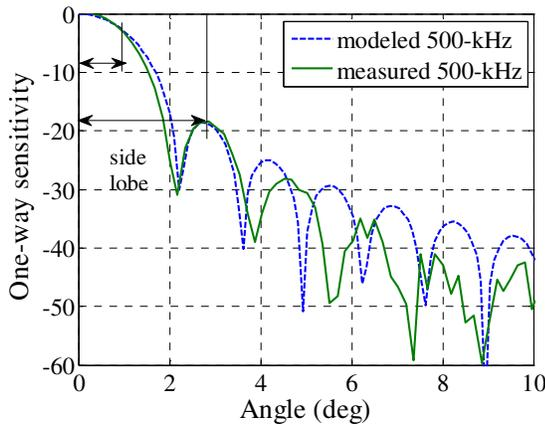
Figure 4: Comparison between modeled and measured shaded transducer beam patterns. Solid line corresponds to measurements collected at the TRANSDEC test facility, San Diego, CA. Dashed line depicts beam pattern computed using numerical model (Eq 3) with the following parameters:  $F_0=500$ -kHz,  $d=120$  mm,  $C=1500$  m/s.
