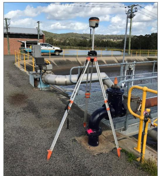
Fig. 2. Hemisphere S321 Smart Antenna.
