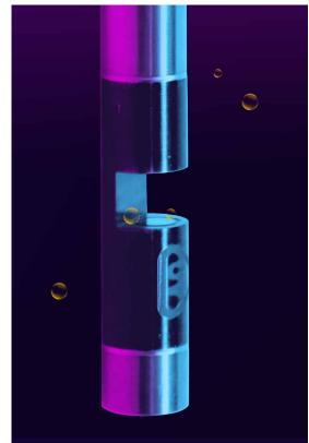
Ensure that there are no bubbles accumulating on the sensor faces, as these can affect readings.
