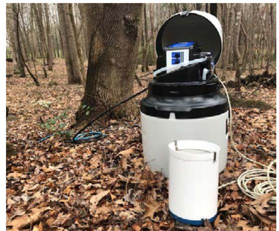
Figure 1: ProSample PM-12 and H-3401 rain gauge
