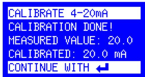
**\*\*\*TROUBLESHOOTING TIP:** If the measured value during the 20 mA calibration does not stabilize, there is not enough power running through the current loop and additional power needs to be inserted into the loop, or a charging system like a solar panel and regulator needs to be connected to the system if an appropriate battery size has already been installed.
