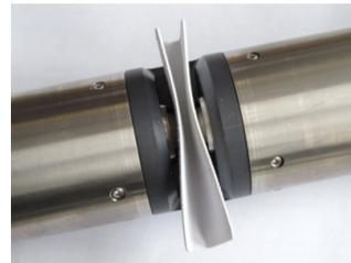
Manual cleaning of a UV probe is recommended every 5 to 7 days
