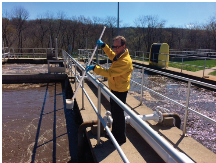
Figure 2. Dr. Rob Smith using a sample dipper to collect a representative sample from the biological tank.
