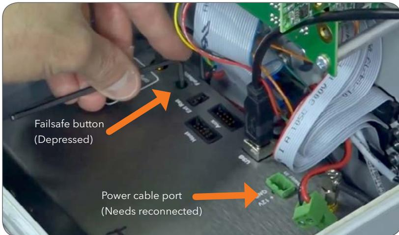
**6** Press and hold the **Failsafe button** while reconnecting the power cable to the terminal on the transmitter (should feel a click when depressed). After power has been reconnected, release the Failsafe button.
