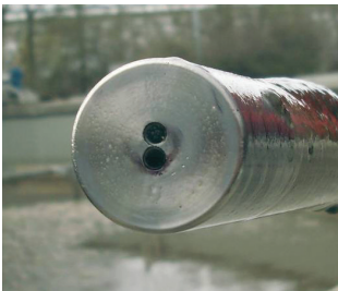
A ViSolid sensor with UltraClean technology remains clean after a 30-day deployment.
