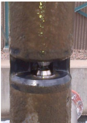
A 5 mm gap YSI UV sensor deployed after one week with UltraClean® technology. No fouling observed on optics.
