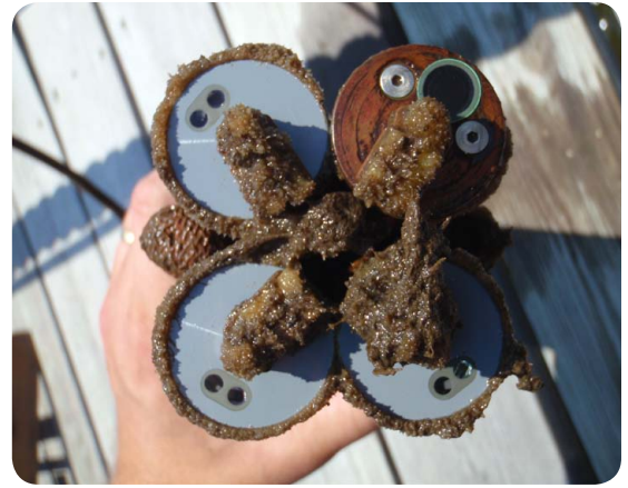
Copper tape, copper-alloy sensor guard and mesh screen would provide additional anti-fouling protection to the equipment above and at left.
