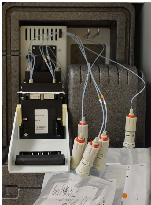
figure 5-20 Absorbent paper in the receptacle of the MultiPort valve
