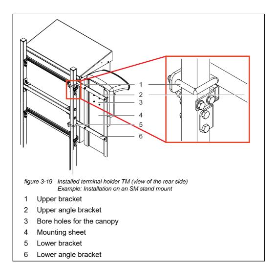
Preparing the mounting stand or rail mounting accessory for the terminal holder The terminal holder is installed at the left-hand side of the Alyza IQ. Thus the terminal is always visible, even with maintenance activities being executed at the open housing of the Alyza IQ.
