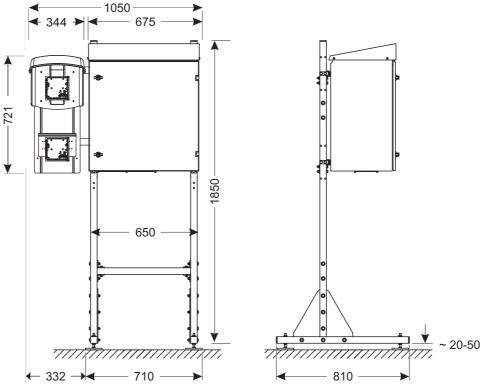
figure 8-2 Dimension drawing of Alyza IQ, installation on a mounting stand (dimensions in mm)
