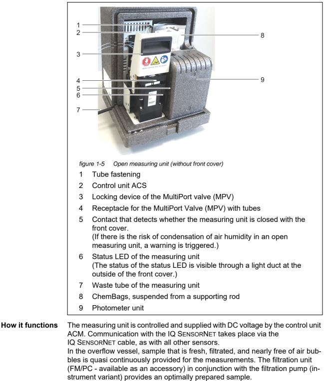
A syringe pump in the measuring unit makes all the liquids move (sample, reagents, standard solutions, cleaning solutions). The MultiPort Valve (4) runs each of the moving liquids to the place where they are required. The dosing of the reagents to the sample takes place in the mixing chamber in the MultiPort valve.
