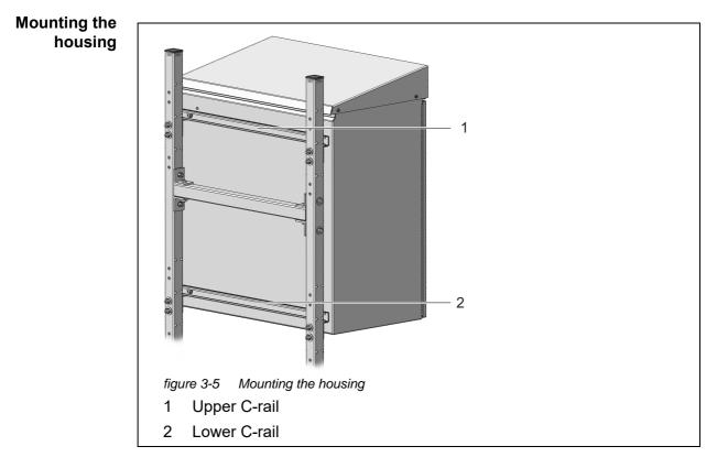
9 Mount the housing by hooking the C-rails (1 and 2) fixed on its rear side into the four retaining hooks of the stand mount.
