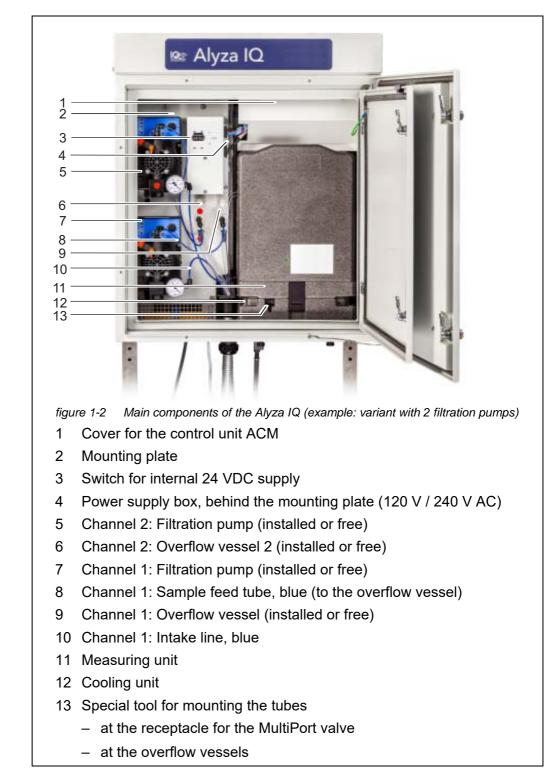
**Instrument design** fig. 1-2, 10 shows the main components of the Alyza IQ.
