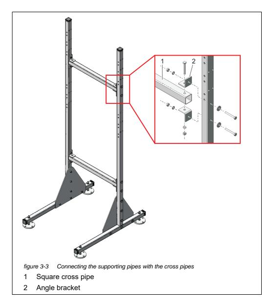
5 Connect both supporting pipes with each other using the two square cross pipes (1). For each joint, use two angle brackets (2), three hexa-gon head screws, two large plain washers, three spring washers and three locknuts.
