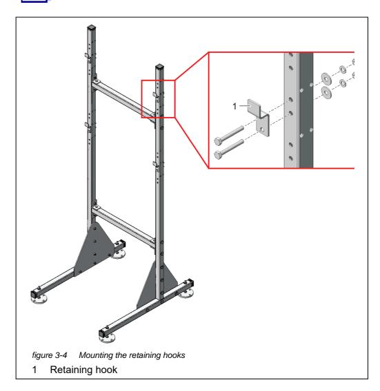
6 Mount the four retaining hooks (1) on the supporting pipes. For each hook, use two hexagon head screws, large plain washers, spring washers and locknuts.
