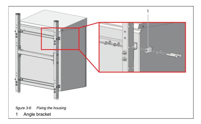
10 Fix the housing on both sides with four brackets (1) so it cannot shift sideways. For each bracket, use two hexagon head screws, small plain washers, spring washers and locknuts.
