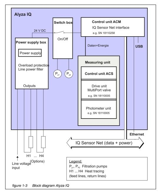
**Operation** The Alyza IQ is connected to the IQ SENSORNET via the IQ SENSORNET cable (SNCIQ) connected to the control unit ACM and conducted to the outside. The Alyza IQ is operated with a terminal on the IQ SENSORNET. If maintenance activities are being carried out on the open Alyza IQ, a terminal for operation must be installed or docked in the vicinity of the Alyza IQ.
