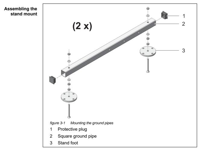
1 Press the plastic protective plugs (1) into both ends of the square ground pipes (2).
