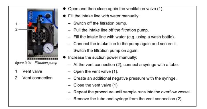
6 As soon as a sufficient amount of sample is flowing, reduce the pump capacity as far as possible (to approx. 2 - 10 %) with the rotary knob.
