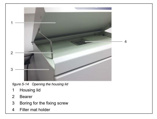
3 Open the upper filter mat holder with the aid of a screwdriver by levering it off and exchange the upper filter mat (see fig. 5-15,  $\square$  137).
