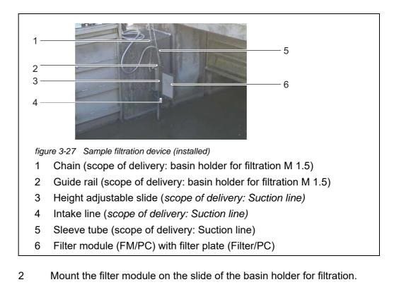
3 Connect the intake line to the filter module.
