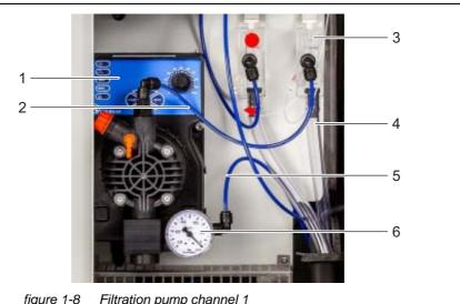
figure 1-8 Filtration pump channel 1
