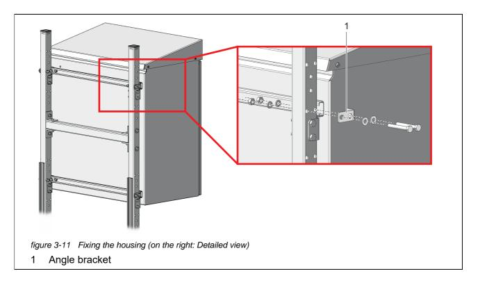
8 Fix the housing on both sides with four brackets (1) so it cannot shift sideways. For each bracket, use two short hexagon head screws, small plain washers, spring washers and locknuts.
