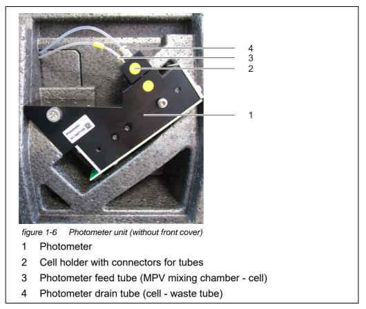
The photometer unit has an LED as the light source and a photo diode as the detector. After the measurement, the liquid is removed from the photometer unit through the waste tube (4).
