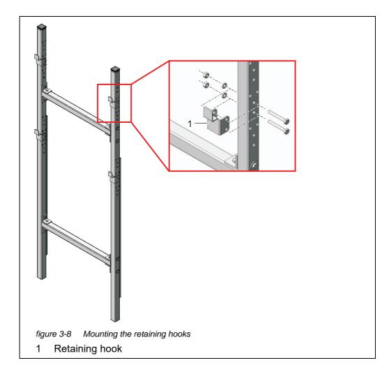
3 Mount the four retaining hooks (1) on the supporting pipes. For each hook, use two short hexagon head screws, spring washers and lock-nuts.
