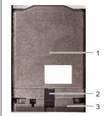
figure 6-4 Fixing the measuring unit
