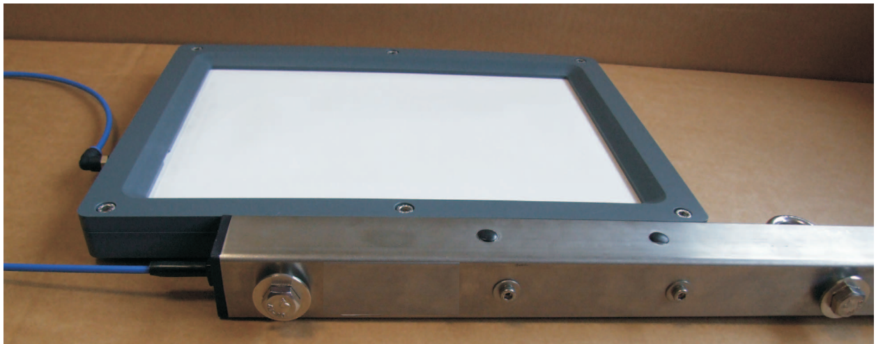
Bild 4-1 Filtration unit (filter module mounted on the guide slide)
