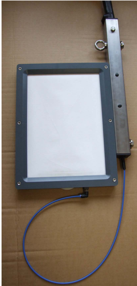
Bild 4-2 Filtration unit (filter module mounted on the guide slide)
